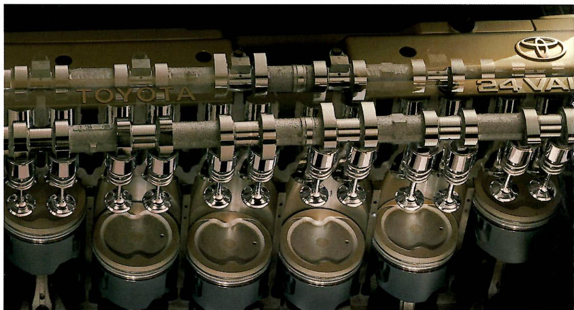
■ 4.2-litre OHC diesel engine is powerful yet quiet and produces high output and torque as well as providing improved durability. 4.2 litre Diesel (1HZ) 96kW/4000rpm 280Nm/2000rpm —SAE net—
